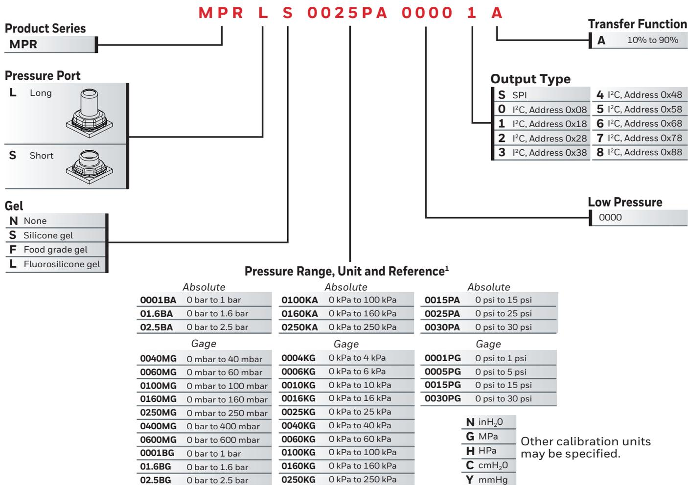
The MPR series is available in a number of configurations. Contact Honeywell or your authorized distributor for a current list of available configurations. For applications above 250,000 units per year, additional configurations are available.
